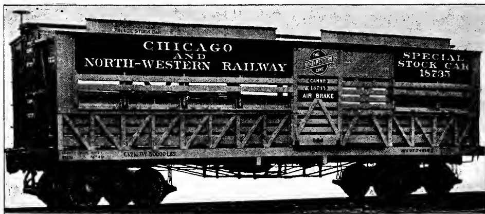
Fig. 39. STOCK CAR FOR CATTLE AND HORSES. CHICAGO & NORTHWESTERN RAILWAY. Capacity, 50,000 lbs. Weight 34,550 lbs. Arrangements for Feeding and Watering, End Doors for Loading Lumber and Rails, and Equipped with Air Brake and Swing Motion Truck.
